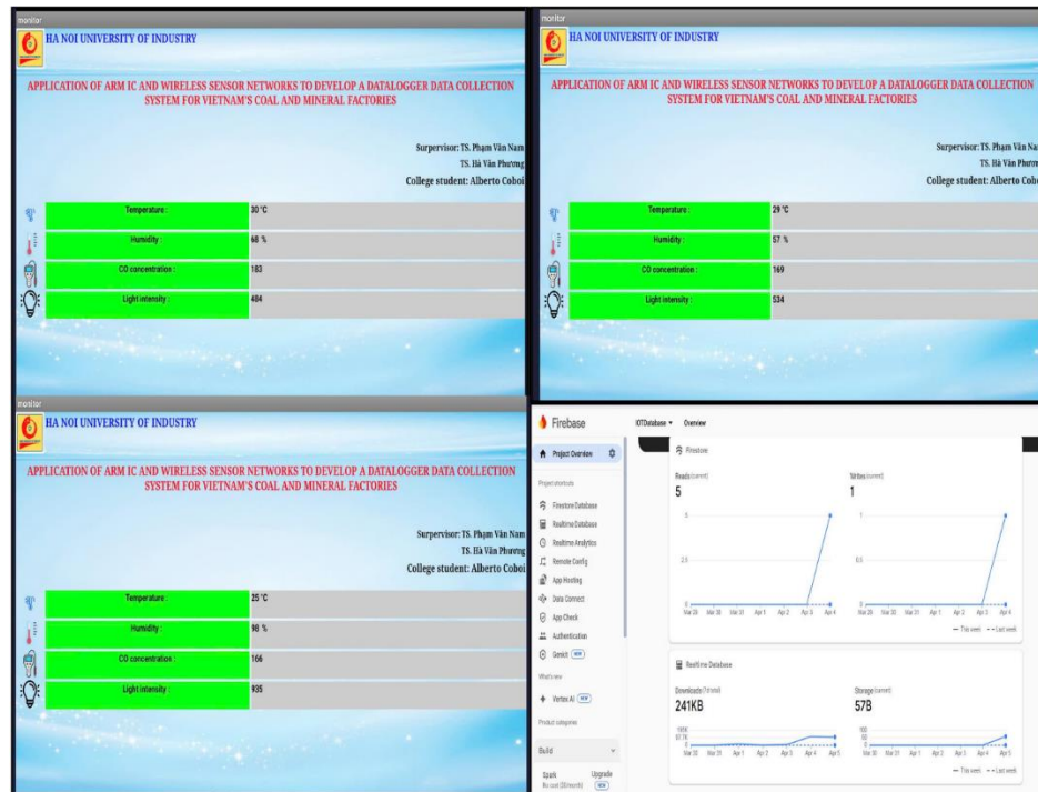
Figure 4-3: Using an app interface, temperature, humidity, CO2, and light intensity were monitored over the course of three distinct experiment days. A lines chart displaying the values of the data stored in Firebase is also included.
