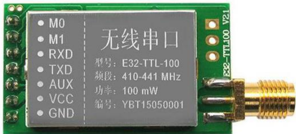
Figure 3-12: The E32-TTL-100 SX1278 LoRa Module.
