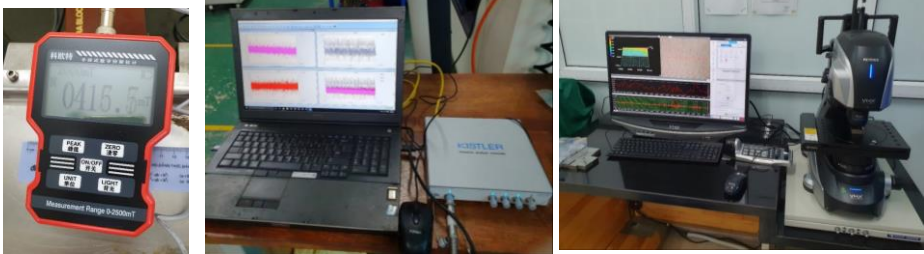
Fig. 3.2 Magnetic field measuring devices KT-101, Kistler 9139AA and VHX-7000
