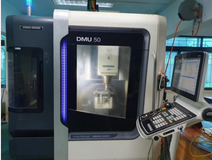
Fig. 3.1 Image of experimental equipment for polishing Ti-6Al-4V alloy MRF on 5-axis CNC machine DMU50
