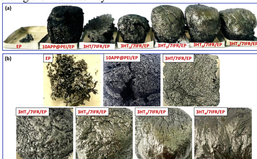
Figure 3.36. Photographic images of the char layers of EP and its composites after combustion at 900 °C: Side view (a) and Top view (b)
