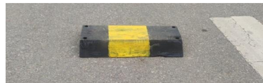
b. Pulse-shaped profile bumps are installed on the test track
