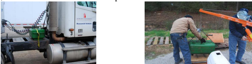
Figure 4.1. How to measure fuel consumption in a road-driving vehicle according to SAE J1321 standard.
